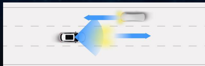
Switch to low beam for oncoming vehicles
