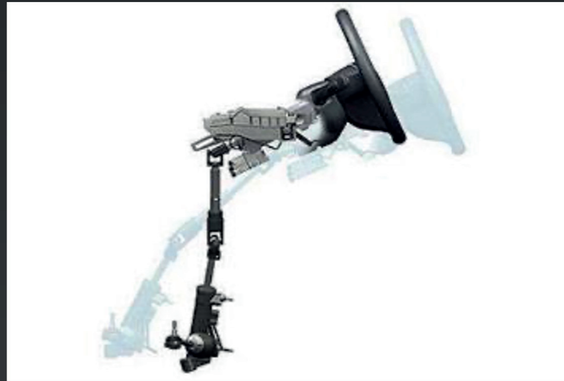
Collapsible Steering Column
